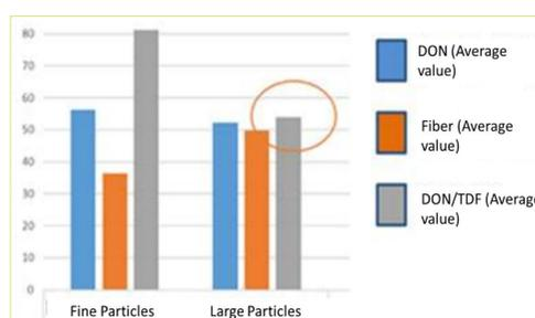
Effect of Hammer Mill system vs Large/Fine particle size Fractioning configurations
