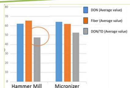
Deoxynivalenol content, fibre content and ratio deoxynivalenol to fibre, obtained with Hammer Mill and Micronizer
